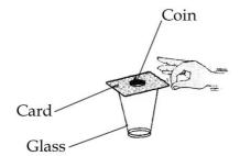
In the above experimental set-up, a student given the card a sharp, fast horizontal flick with a finger.
